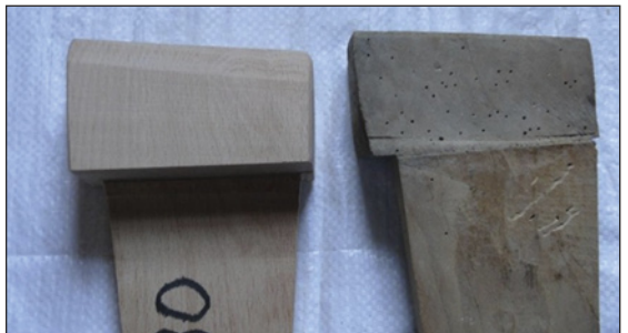
comparison between the new and original 100 year old cogs
