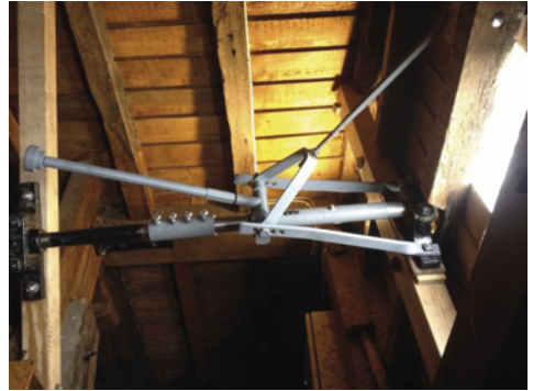
Hammond Sweep governor clutch mechanism as fitted in the mill
